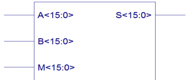
Figure 4: View Technology Schematic of 16-bit Reversible Residue sub-tractor using TSG Gate
