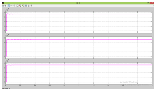
Figure 20 Reactive Power output from the STATCOM device fed into the grid at bus B2
