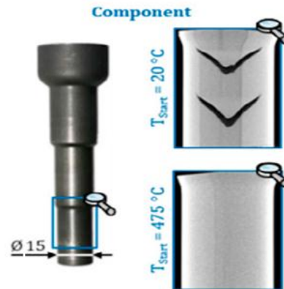
Figure 6 (b) Shape of the formed part and computer tomographic image of cold and warm formed
