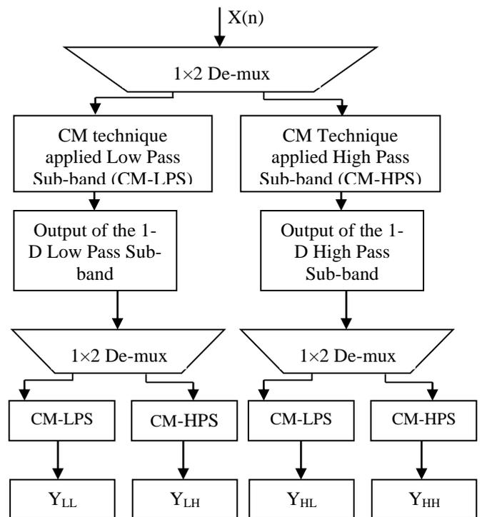
Figure 2: Block Diagram of 5/3 2-D DWT using CSD Technique
