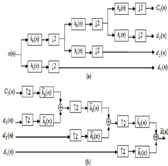
Figure 1: Three level decomposition of an image
